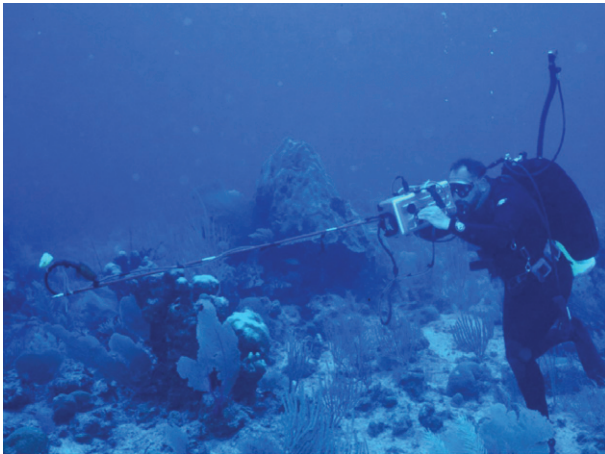
Figure 3 Recording sound and video underwater using a hydrophone mounted on a boom. Photo by Lisa Kerr Lobel. Reproduced from Lobel PS (2001) Sounds produced by spawning fishes. Marine Technology Society Journal 35: 19–28.
